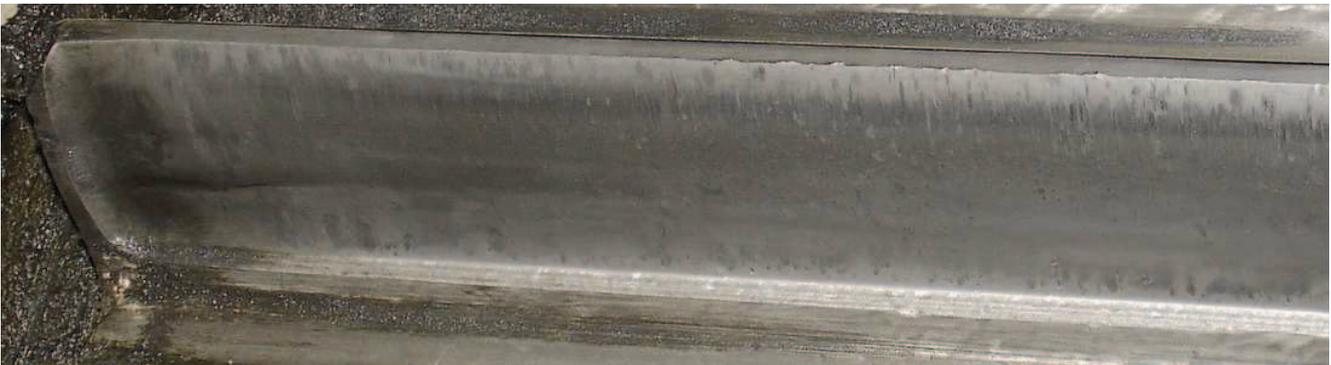
Examples of teeth needing to be cleaned (images above) and of the effects of abrasion on working flanks (lower image).
