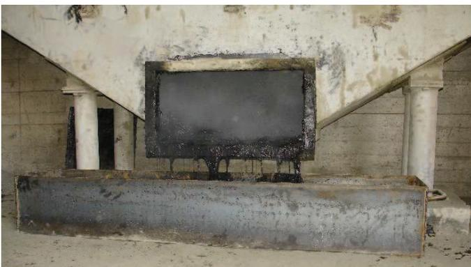
Example of a used solvent evacuation tank.
