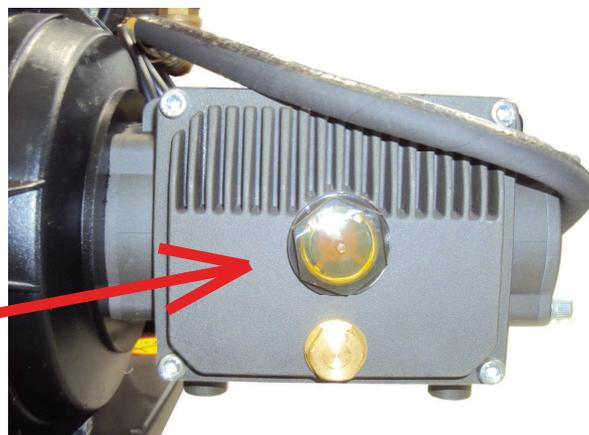
The oil level must always be above the reference mark on the dipstick (use oil type SAE 20/30).
