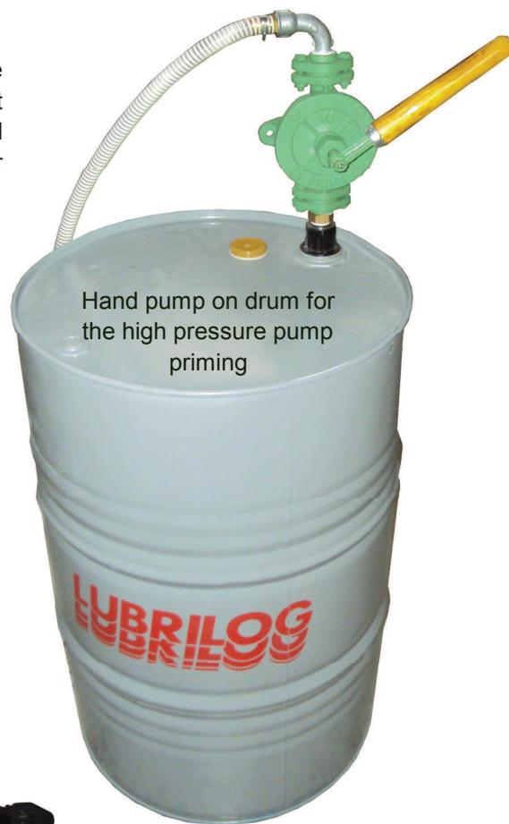
Hand pump on drum for the high pressure pump priming
