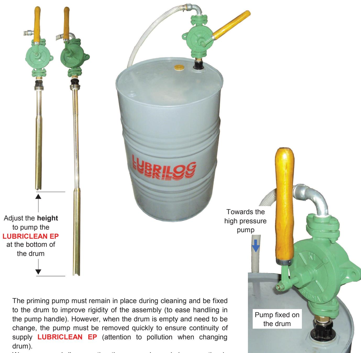
The priming pump must remain in place during cleaning and be fixed to the drum to improve rigidity of the assembly (to ease handling in the pump handle). However, when the drum is empty and need to be change, the pump must be removed quickly to ensure continuity of supply **LUBRICLEAN EP** (attention to pollution when changing drum).
