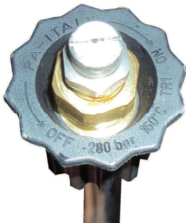
The spray nozzle must be adjusted to obtain a jet with the greatest intensity even during the initial cleaning (during this phase, the operator can distance the nozzle to spray a more diffuse).
